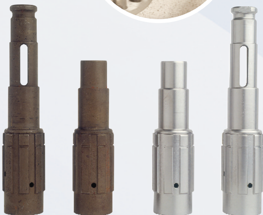
Before and after samples of the surface finish using the Vixen Jetair machines
